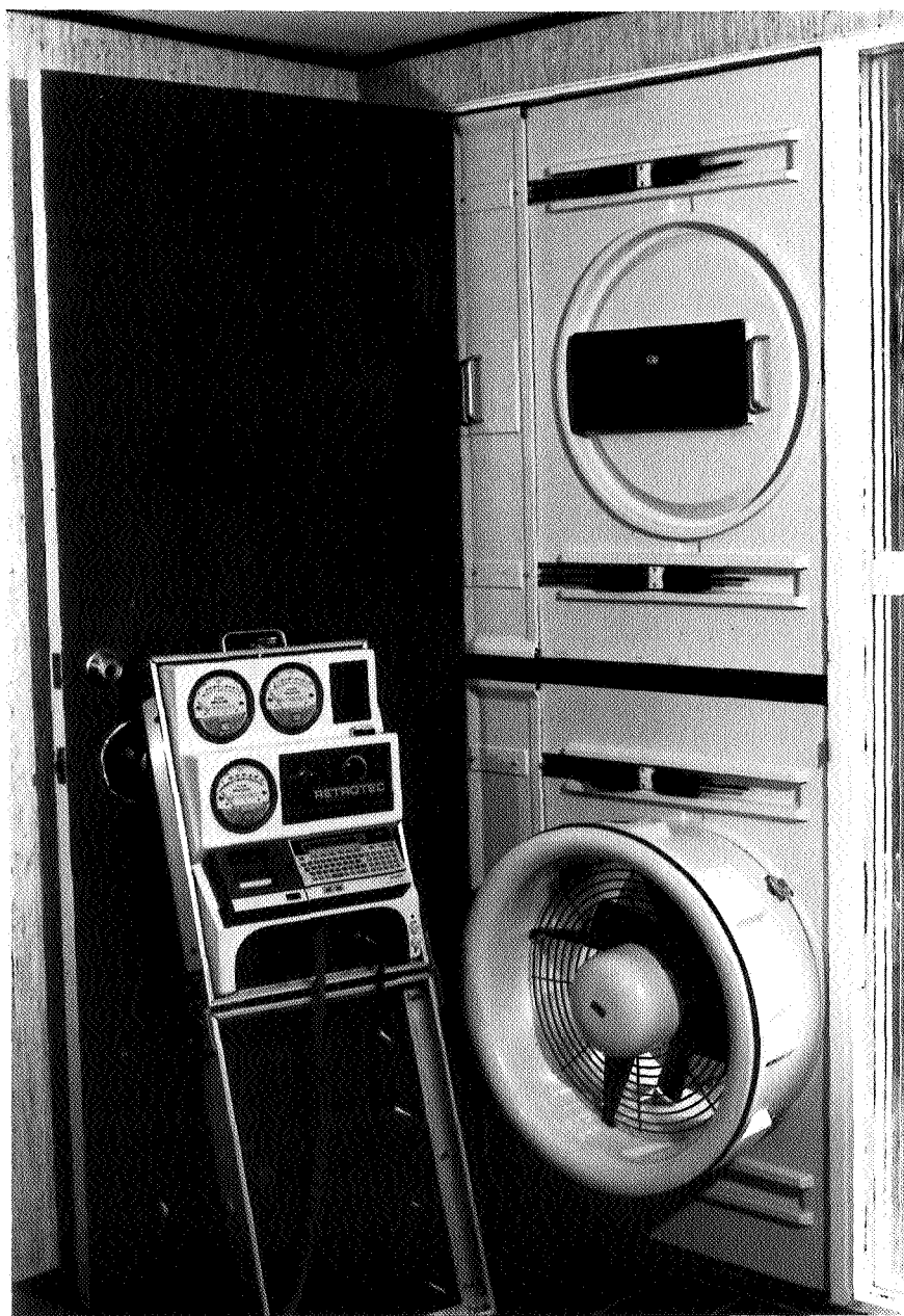
Figure 4.3.1 Blower door. Modular panel type. Retrotec (see Table 4.3.1)
