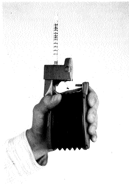
Figure 6.3.1 Detector tube and bellows for carbon dioxide sampling
